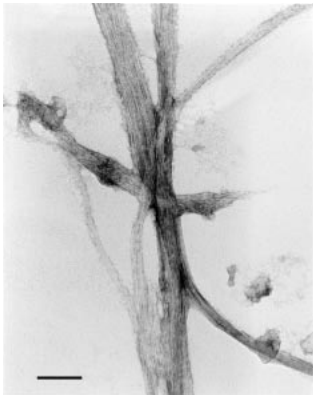
Fig. 1 Transmission electron micrograph (using negative staining technique with uranyl acetate solution) of polymer mesofibres supported on a carbon film. Magnification bar = 100 nm.
